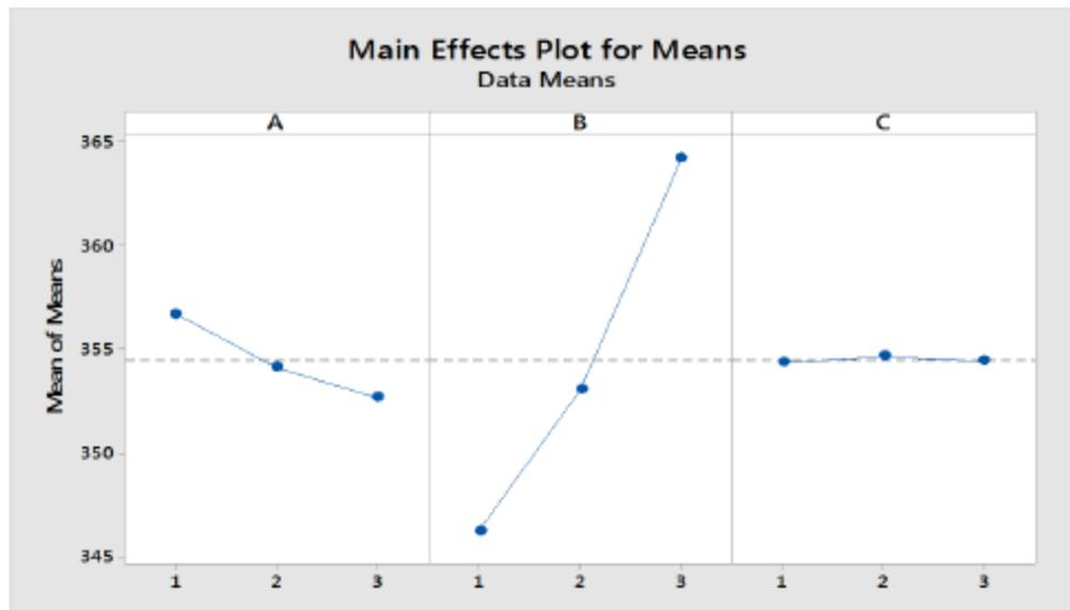
Main effects plot for hardness is shown in Fig. 6. The first plot displays effect of current on hardness using data means. The graph shows that the hardness decreases rapidly as current increases from 121 amp to 139 amp.
