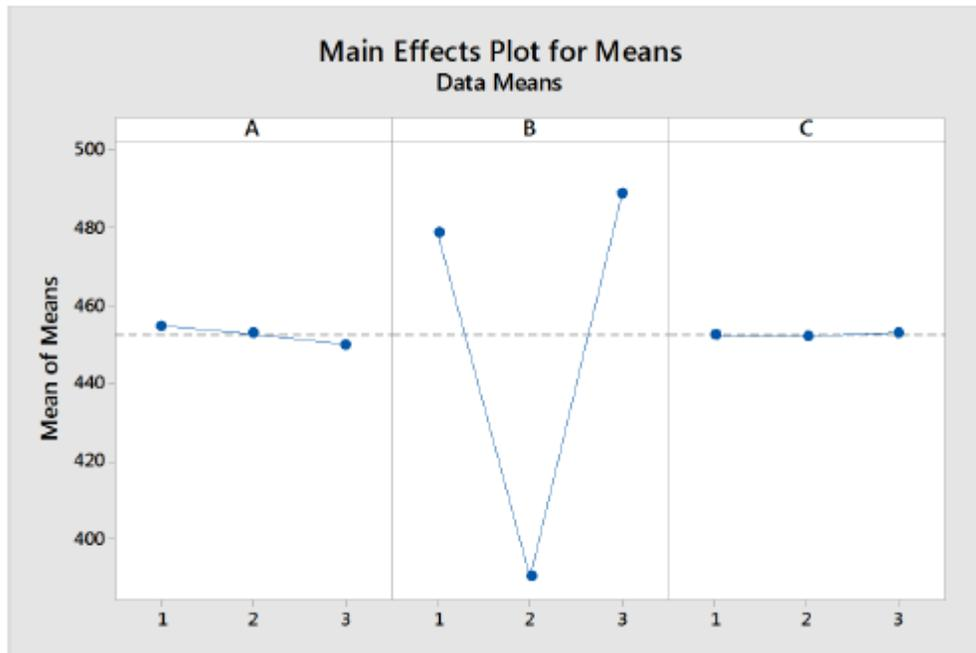
Main effects plot for UTS is shown in Fig. 9. The first plot displays effect of current on UTS using data means. The graph shows that the UTS decrease rapidly as current increases from 121 amp to 139 amp.
