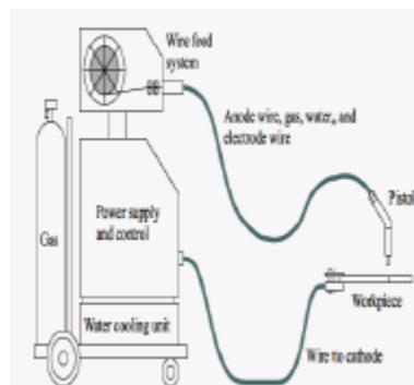
MIG welding is useful because you can use it to weld many different types of metals: carbon steel, stainless steel, aluminum, magnesium, copper, nickel, silicon bronze and other alloys.
