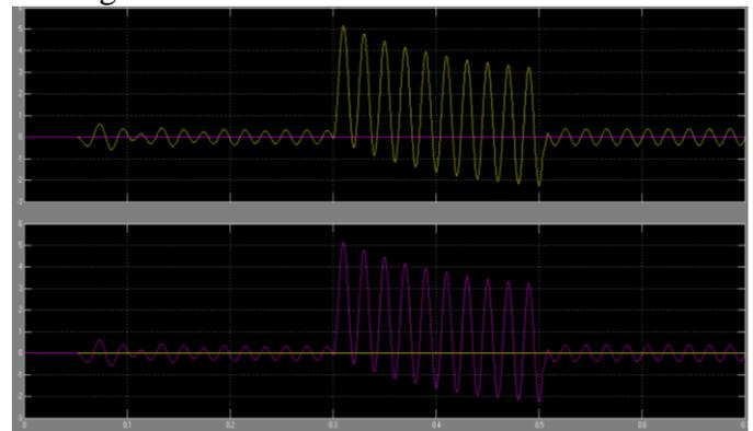
Fig-2 Simulation for Inrush & Fault Current
