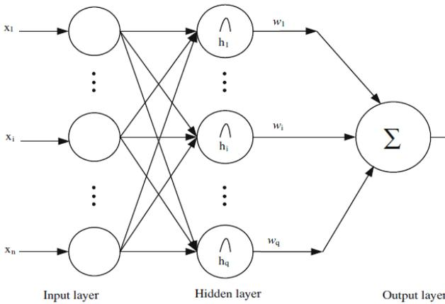
Fig. 2. Typical radial basis function neural network architecture.
