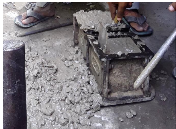
Figure 2 pouring the concrete into the moulds and compacting them thoroughly
