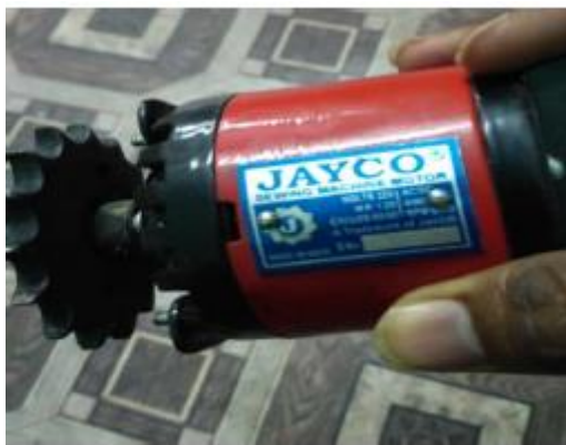
Sewing Machine Motor: 220V, 230W, 7500 rpm
