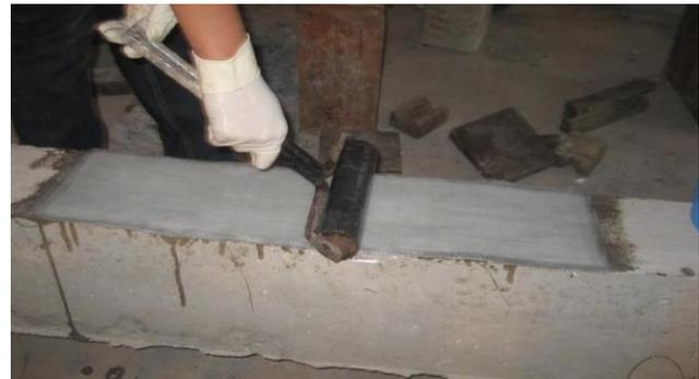
Fig. 3.5 Roller used for the removal of air bubble
