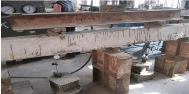
Fig. 3.14 Experimental Setup of the Beam
