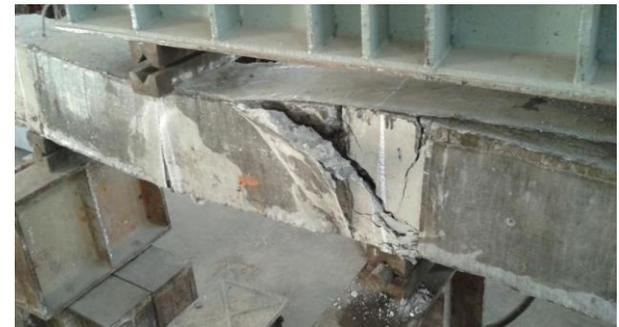
Figure 3.18 Ultimate failure of beam by debonding of FRP with concrete Cover
