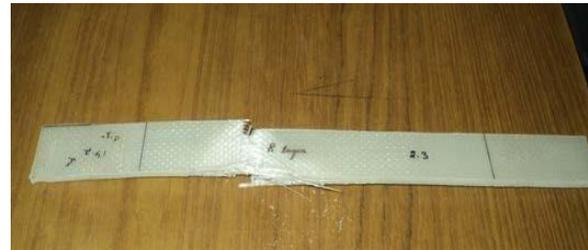
Figure 3.10 Specimen failure after tensile test
