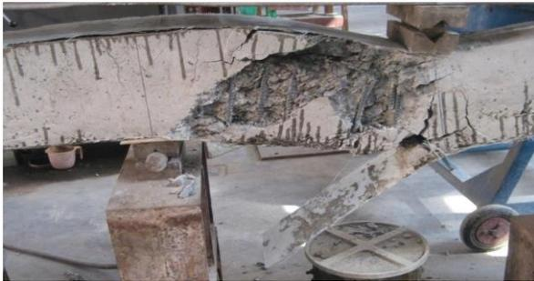
Fig. 3.16 Magnified view of the failure of the beam
