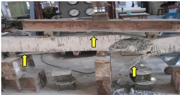
Fig. 3.15 Deboning failure of FRP
