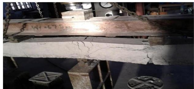
Fig. 3.13 Control Beam, CB2 after failure
