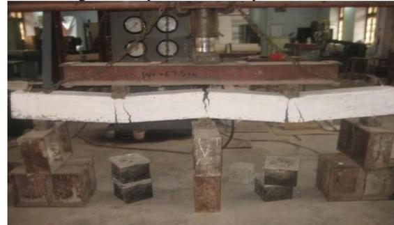
Fig. 3.12 Flexural failure of CB1
