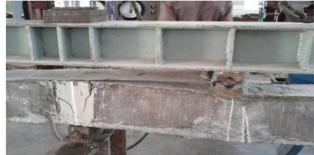
Figure 3.17 Tensile rupture of FRP at mid section of right span at lower value of load
