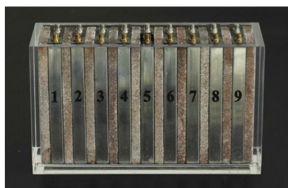
Figure 5: Battery pack design (a) using the copper foam-paraffin composite.
