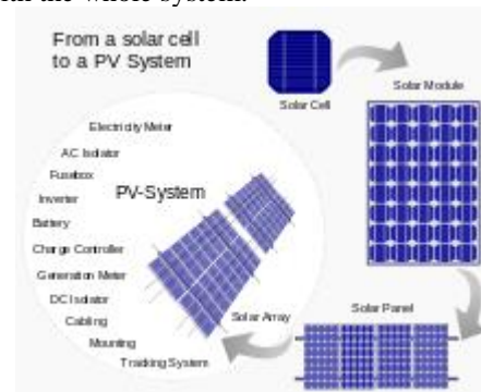
Fig 1: Diagram of the possible components of a photovoltaic system
