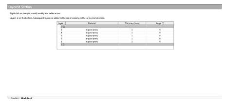
Figure: Layering with e glass Epoxy as material
