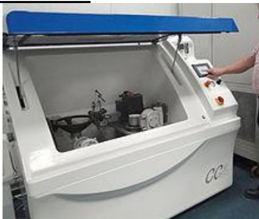
A modified salt spray chamber in use
