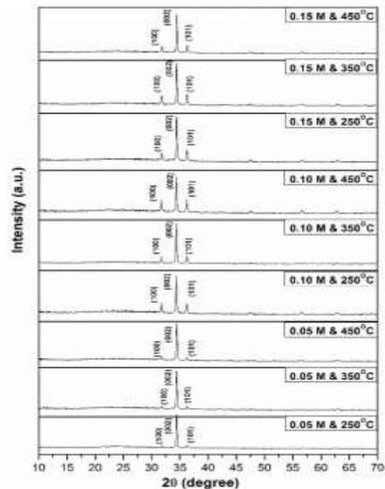
**Fig. 1. The XRD pattern of ZnO thin films for different mole concentrations and annealing temperatures**
