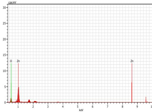
Fig. 3. The EDX spectrum of ZnO thin films for 0.10 M with annealing temperature of 450°C
