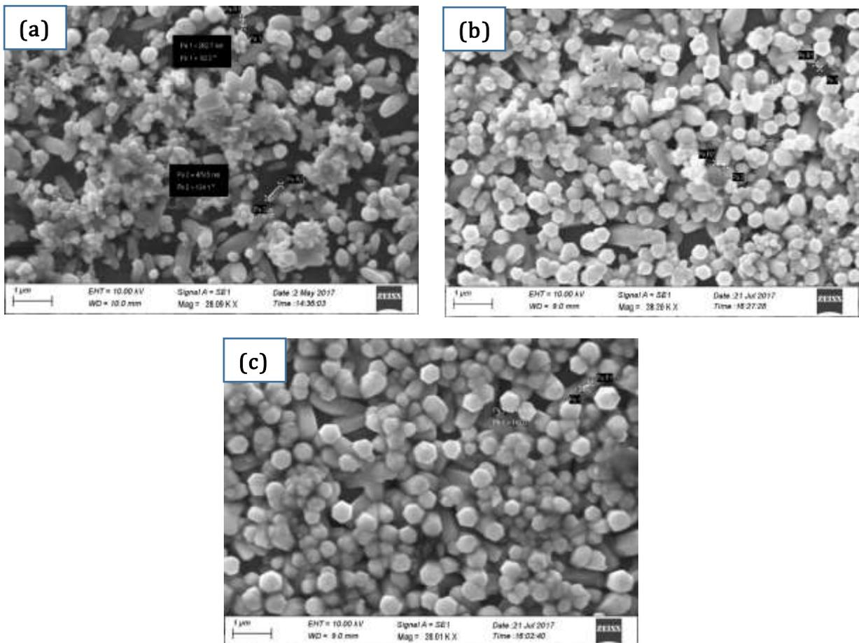
Fig. 2. The SEM images of ZnO thin films for different mole concentrations of (a) 0.05, (b) 0.10 and (c) 0.15 M at annealing temperature of 450°C
