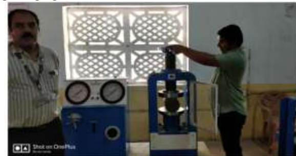
Fig 10 Split Tensile Strength Of Cylinder Fixed To Machine
