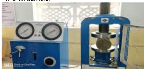
Fig4.6: Split tensile test of cylinder
