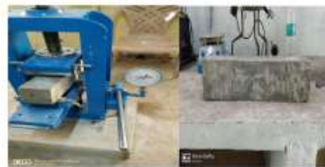
Fig4.7: Flexural strength test on beam, The above figure shows a universal testing machine
