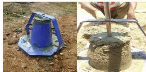
Fig.3: Slump Cone Test Above figure shows a Slump Factor of Fresh Concrete
