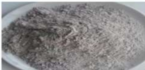
Figure 6: GGBS Used for Concrete Mix
