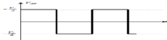
1.7 Output waveform of Half Bridge Inverter
