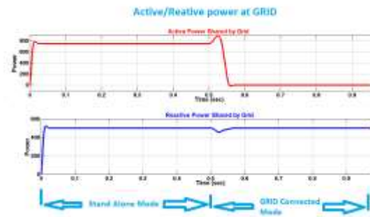
Figure 0-5 Active Power and Reactive Power at Grid
