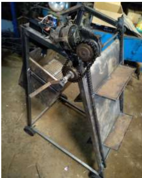
Figure1: mechanical semi-automatic drainage cleaning system.
