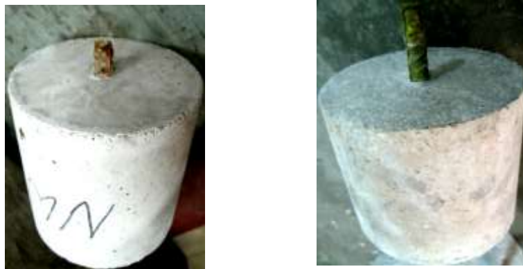
Figure 2. As-received (left) and epoxy paint coated (right) steel bars in cast concrete blocks.
