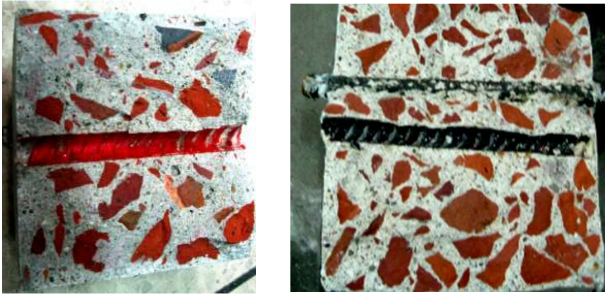
Figure 7. Retained enamel (left) and ujala paint coating layers on the bar-concrete interfaces.
