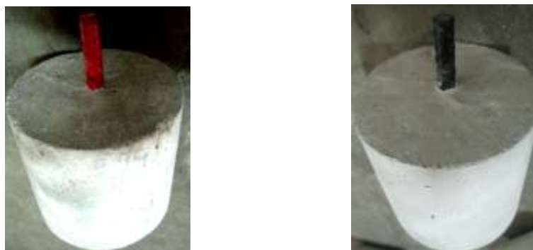
Figure 2. As-received (left) and epoxy paint coated (right) steel bars in cast concrete blocks.
