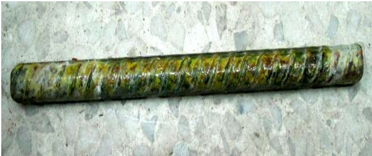
Figure 5. Pulled out epoxy paint coated bar from inside the concrete block.
