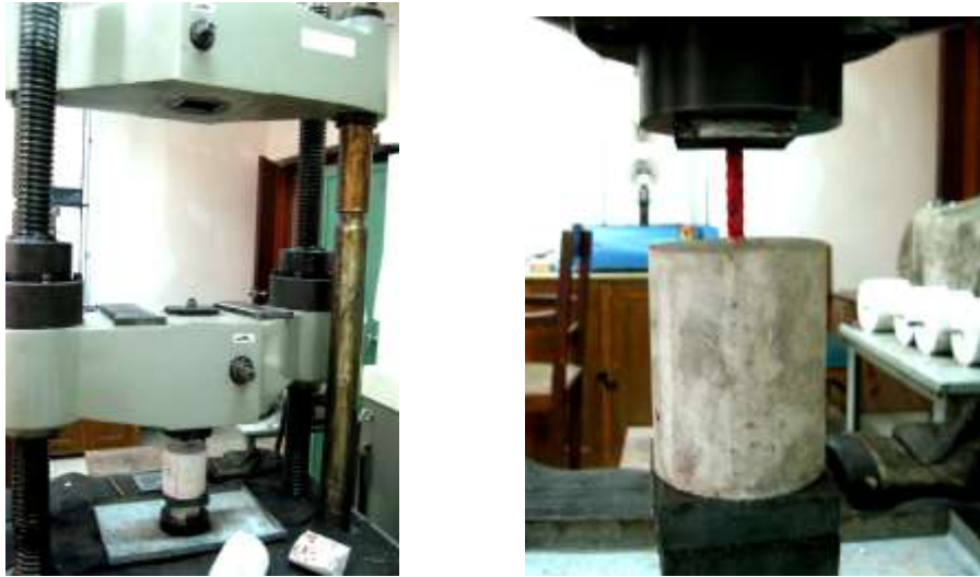
Figure 4. Universal testing machine with special fixture (left) and close-up view of concrete block under test (right).
