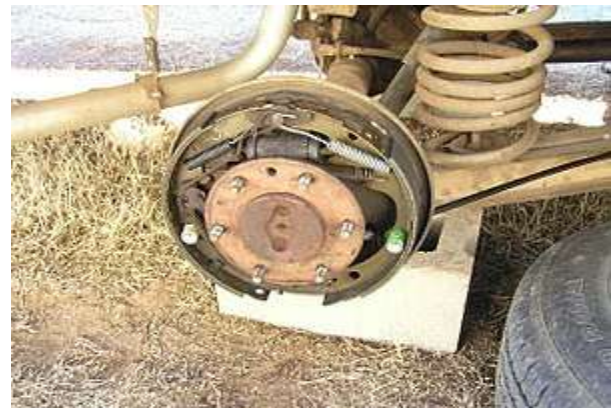
Drum brake with the drum removed, on the rear of Chevrolet pickup truck
