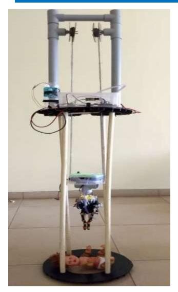
The code was tested and verified using arduino software. The program was successfully uploaded in arduino and input output conditions are verified. The camera module was used and image processing is done using MATLAB. Two 10rpm motors are used for the movement of the robot successfully.
