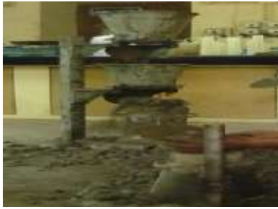
Figure 3.3 Compaction factor of concrete being measured in the Laboratory
