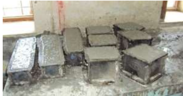
Figure 3.8 Moulds of cement concrete cubes being casted in the Laboratory Phase IV
