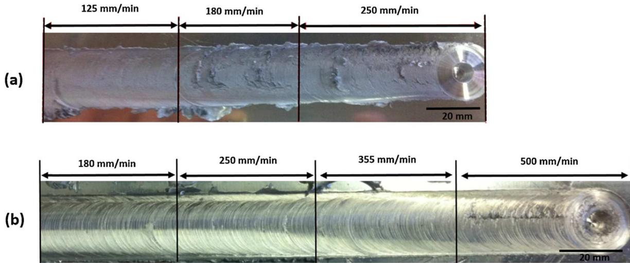
Fig. 20 Comparison of (a) concave and (b) scroll shoulders at increasing welding speed [20]
