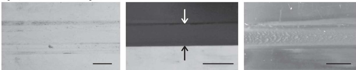
Fig. 23 Effect of traverse speed on the morphology of the weld crown: (a) R1250T50F3.75, (b) R1250T100F2 and (c) R1250T200F3.25 [19]
