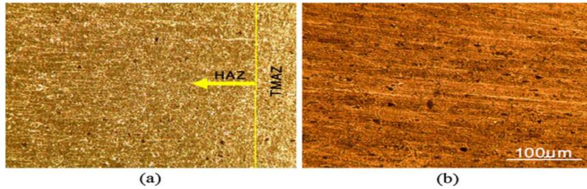
Fig. 11 a the microstructure of TMAZ and HAZ on AA7075 side and b the microstructure of HAZ on AA2024 side [5]
