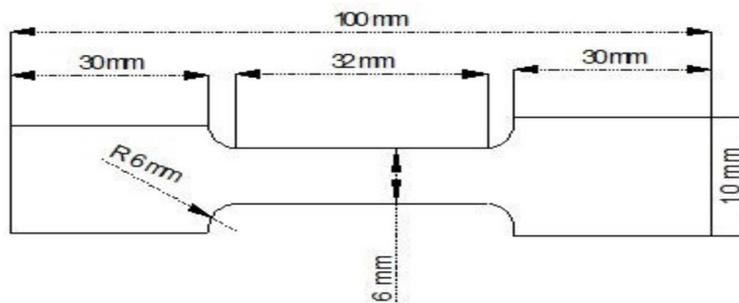
Fig. 14 ASTM E-08 sub size tensile test specimen. ASTM E-08 sub size tensile test specimen.[7]
