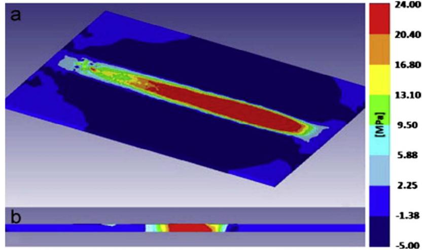
Fig. 7. Longitudinal residual stress distribution (a) on the top surface and (b) in a transverse section of the joint—500 rpm and 225 mm/min case study [16].
