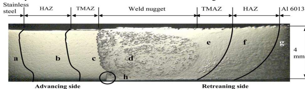
Fig. 16 Macroscopic overview of the cross-section of the friction stir welded Al 6013-T4 alloy to X5CrNi18-10 stainless steel [10]
