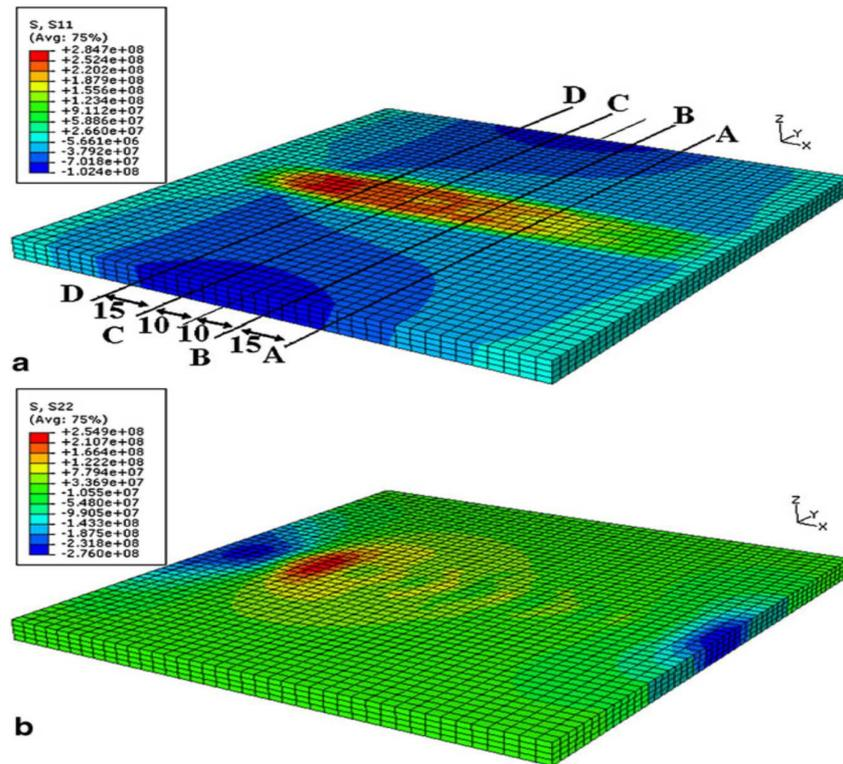
Fig 3. Predicted three-dimensional residual stress distribution in the welded plate. A Longitudinal residual stress and b transverse residual stress ( $v = 280$  mm/min;  $\omega = 1,250$  rpm)
