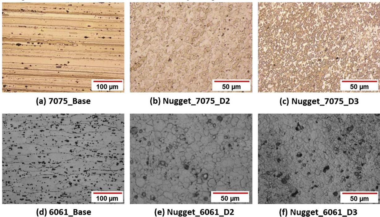
Fig.18 Optical micrographs showing the grain structures of different alloy sub-layers in the nugget zones of the dissimilar welds and the two base metals[12]
