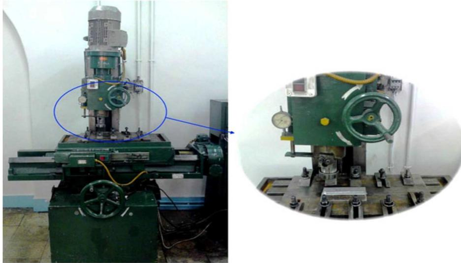
Fig 4. The machine used in the friction stir welding experiments
