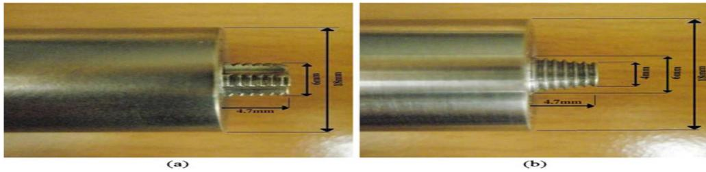
Fig. 9 the geometries of tools (a) threaded 4-flute tool (b) threaded taper tool [5]
