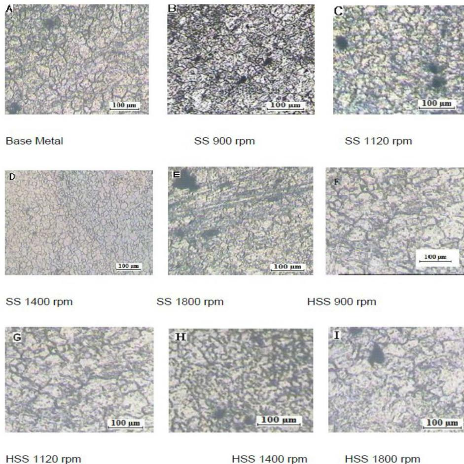
Fig.24 (A-I): Effect of tool material on stir zone Microstructure with SS tool and HSS tool [20]
