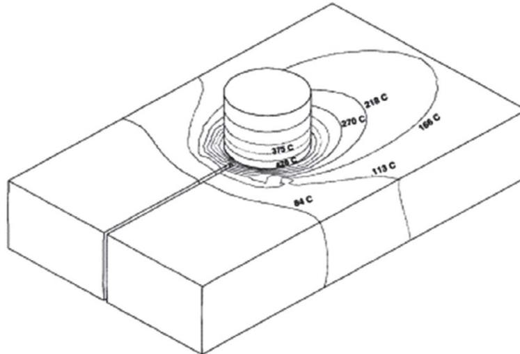
(c) Temperature contours (in °C) on the tool and workpiece surfaces.
