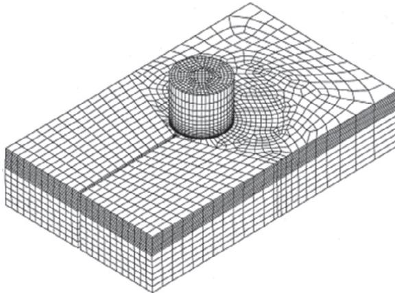
(a) FE mesh of the FSW model enlarged view of the stir-welding tool.
