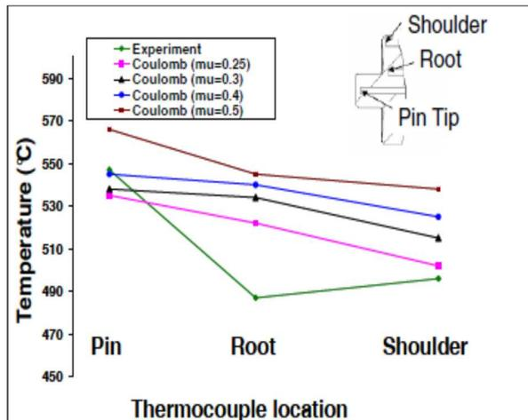
(b) Comparisons of calculated and measured temperature at pin, root, and shoulder locations in the FSW tool with Coulomb friction and the ALE formulation[2]
