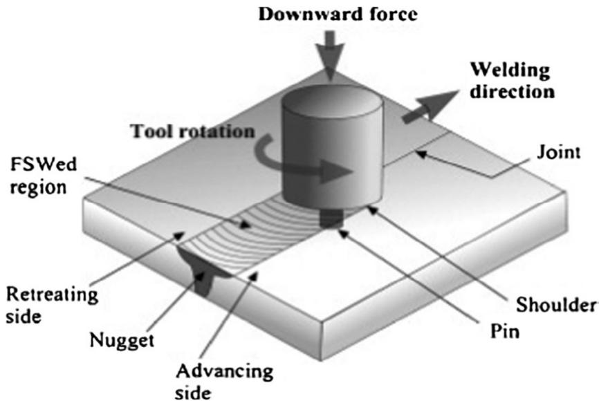
Fig. 1. Schematic drawing of FSW process [1].
