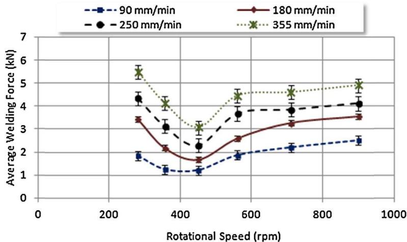
Fig. 21 Welding force with increasing rotational speed [20]
