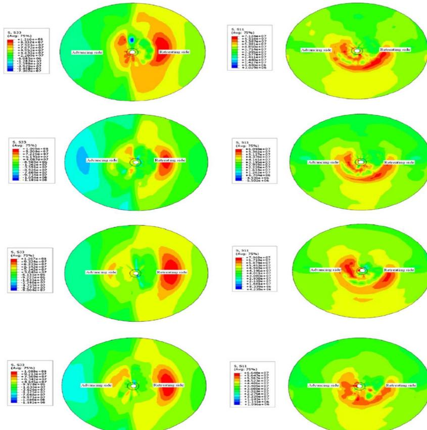
Fig 5. Longitudinal and transverse residual stress profiles for: a sample A, b sample B, c sample C, and d sample D
