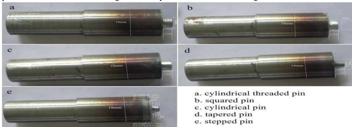
Fig.12 shows the tool diagram used for this experimental work [6]
