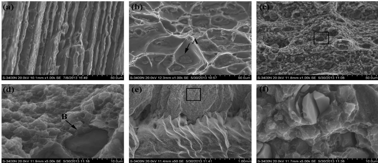
Fig. 22 SEM fractographs of (a) BM, (b) 350 rpm-50 mm/min, (c) 350 rpm-100 mm/min, (d) higher magnification of (c), (e) 650 rpm-100 mm/min, and (f) higher magnification of (e).
