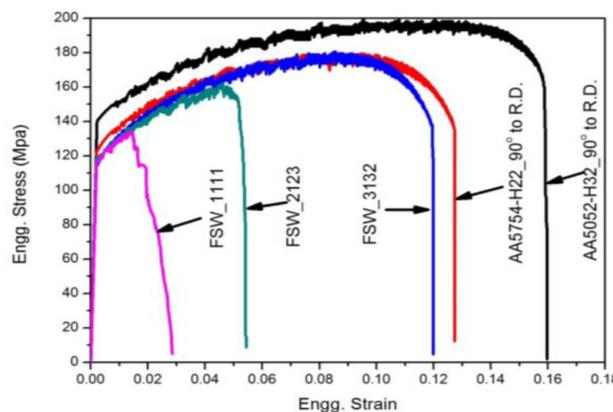
Figure .15. Typical engineering stress strain curves for both BM and TFSWBs [7]
