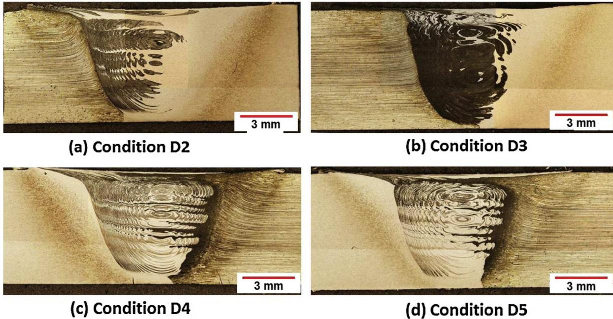
Fig. 17 Macro-views of the cross sections of joints produced under different conditions [12]
