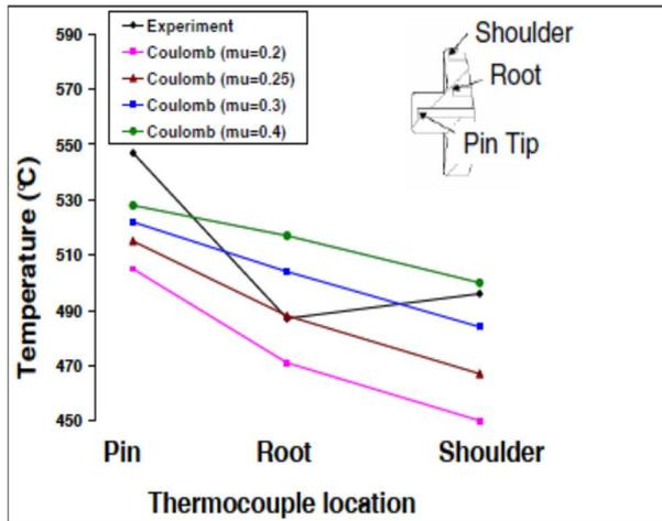
Fig 2(a) Calculated and measured temperatures at pin, root and shoulder locations in the FSW tool with Coulomb friction using an Eulerian formulation[2]
