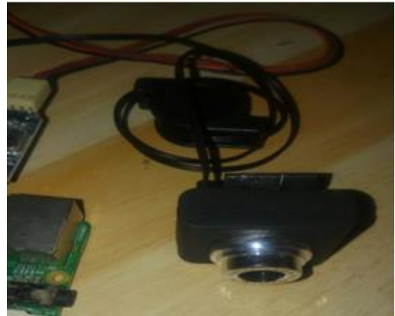
Figure 7: Camera connected to Processor
