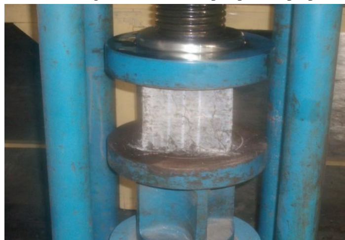
Fig. 1 “Testing of compressive strength test specimen”
