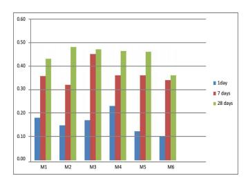
From the above experimental values obtained by the compressive test analysis it is clear that with increase in demolished waste the compressive strength of concrete increase up to M3 mix and the compressive strength will decreases after the increase in demolished waste content in concrete. The sisal fiber usage decreases the compressive strength of concrete as it produces voids and the bond action will be reduced by the smooth texture of sisal fiber.
