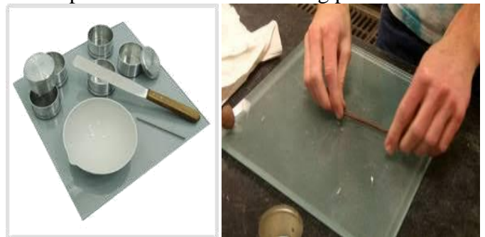
Figure 5: 1) Plastic limit apparatus 2) glass plate Wet weight = 26 gms , Dry weight = 22 gms Final plastic limit value = 19.04%
