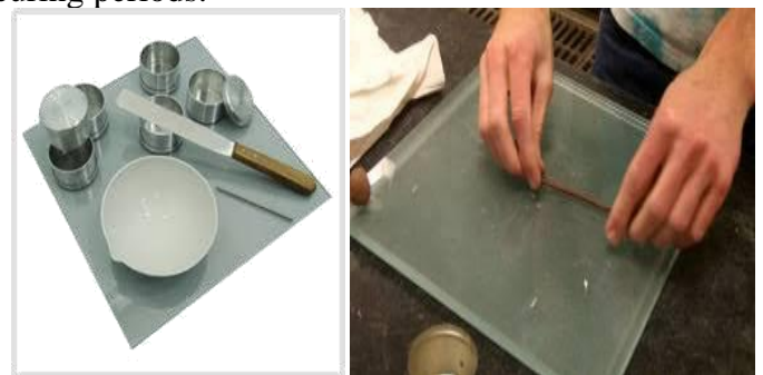
Figure 5: 1) Plastic limit apparatus 2) glass plate
