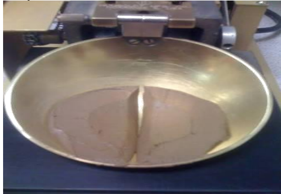
Figure 3: Liquid limit apparatus
