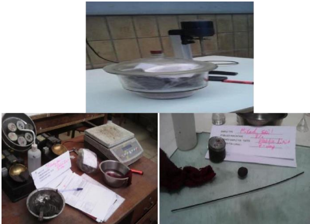
Figure 6: sample curing, Atterberg limit testing
