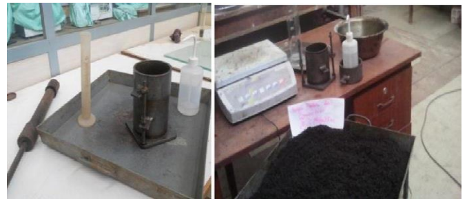
Figure 7: Curing of molasses treated compaction sample, Testing
