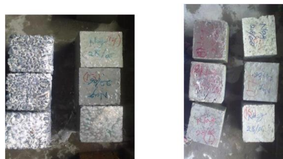
Fig:6. Concrete cubes after acid immersion in H 2 SO 4
