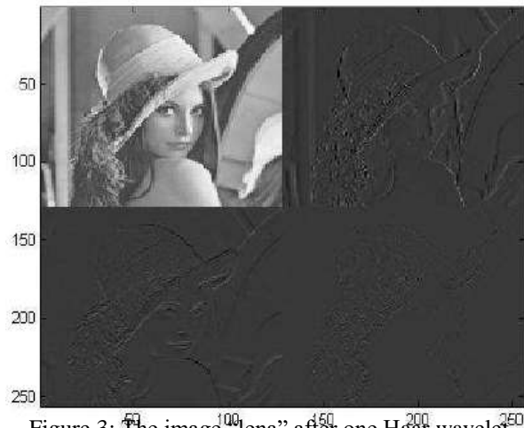
Figure 3: The image "lena" after one Haar wavelet transform
