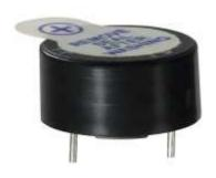
The vibrating disk in a magnetic buzzer is attracted to the pole by the magnetic field. When an oscillating signal is moved through the coil, it produces a fluctuating magnetic field which vibrates the disk at a frequency equal to that of the drive signal.
