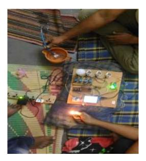
The above figure explains that when the fire has been detected Raspberry Pi processor turns on the water motor.
