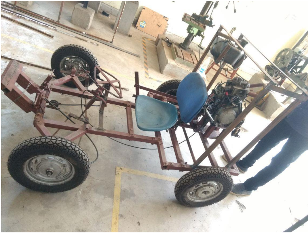
Fig. 9.3 Complete Fabricated Chassis
