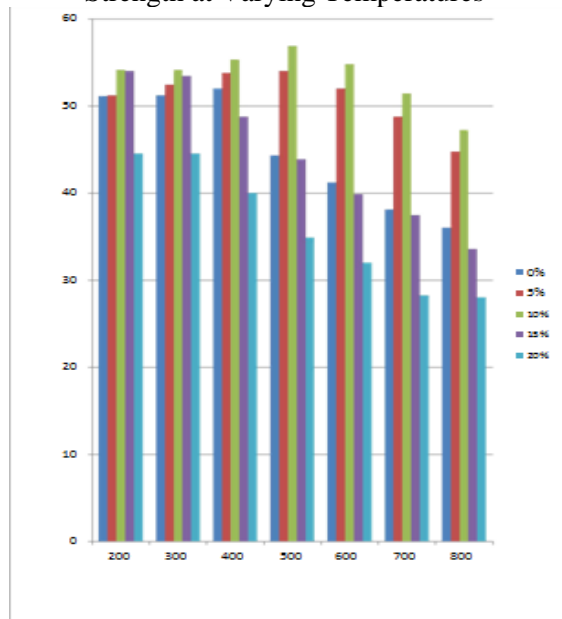
Fig 4.4 M-40 Specimens Compressive Strength at Varying Temperatures
