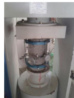
Plate 17: Photograph of Setting of Extensometer
