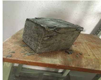
Plate 15: Photograph of specimen after crushing
