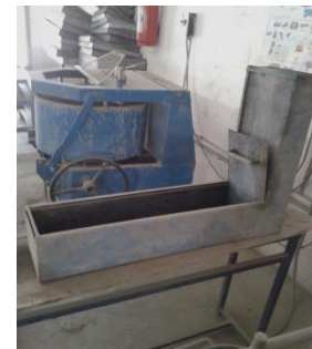
Plate 9: Photograph of L-Box Test on SCC
