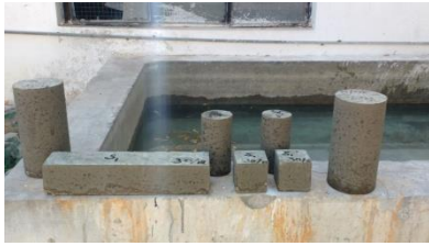
Plate 11: Photograph of dry specimens after curing in curing tank
