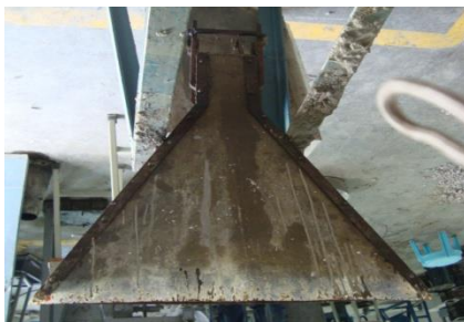
Plate 7: Photograph of V-Funnel Test on SCC
