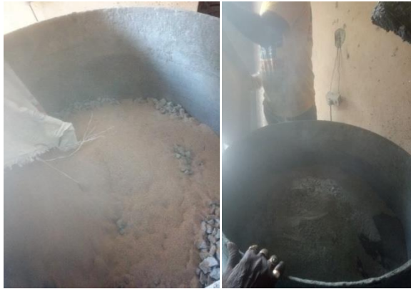
Plate 5: Photograph of dry constituents of SCC with River sand
