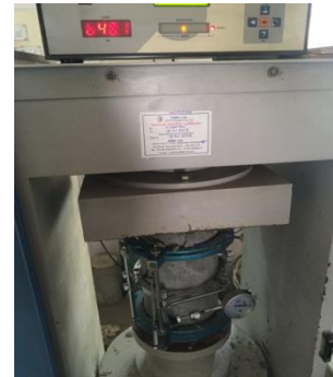
Plate 16: Photograph of Testing of Elastic Modulus by using Extensometer
