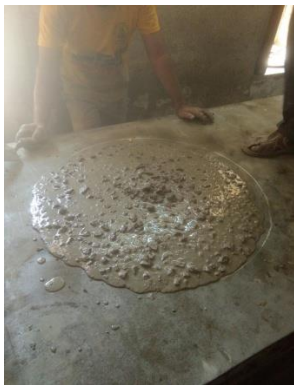
Plate 6: Photograph of Slump Cone Test
