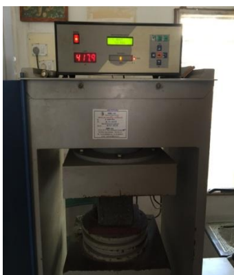
Plate 14: Photograph of Specimen during Compression
