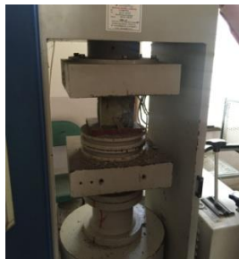
Plate 13: Photograph of Loading Unit of CTM
