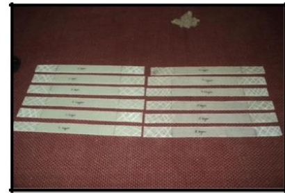
Figure 3-2. Specimens for tensile testing of woven Glass/Epoxy composite
