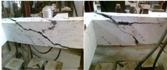
Fig.4.1b Crack pattern at face-1
