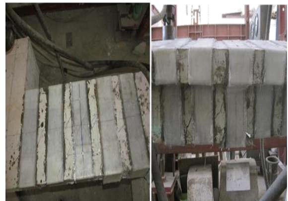
Fig 4.6(a) Fully Wrapped beam after Cracking
