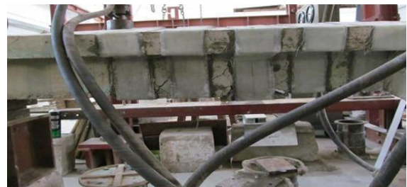
Fig 4.6(a) Fully Wrapped beam after Cracking
