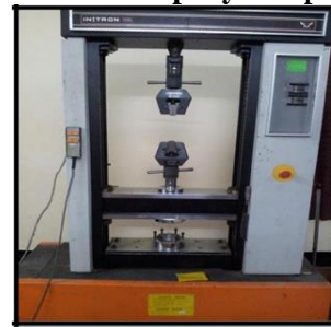
Figure 3-3. Experimental setup of INSTRON universal testing Machine of 600 kN capacities
