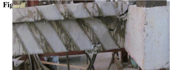
Fig 4.7(a) Beam wrapped with 100mm Bi-directional GFRP (45°) after cracking.
