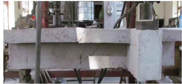
Fig. 4.3 Spiral crack in the beam
