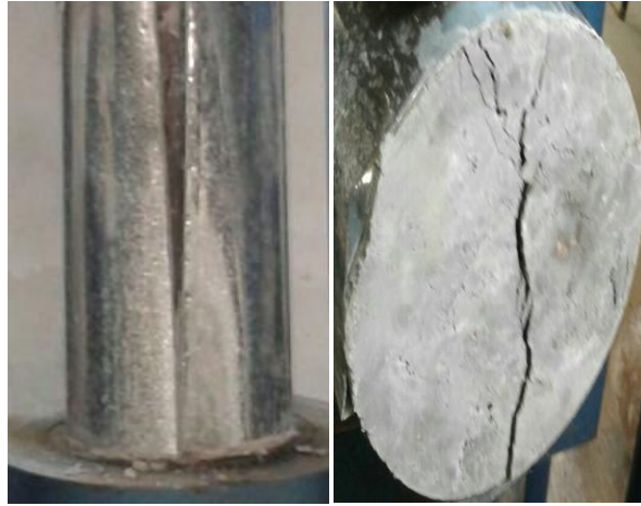
Fig.9. Weld Failure of Geo polymer
