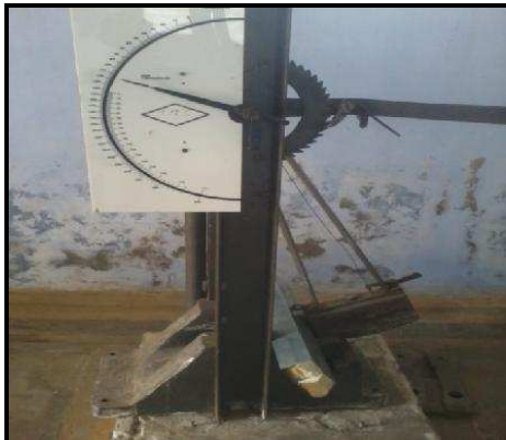
Figure 5 Schematic arrangement of impact test
