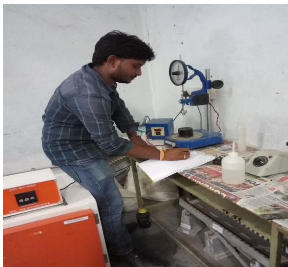
Penetration test in Bitumen sample at Laboratory
