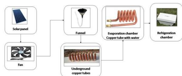
It works by passively drawing in warm ambient air through the funnel, which is fed into a pipe that's been buried underground. This already starts to cool down the air before it's fed into coiled cooper pipe that's been immersed in water in the evaporation chamber. The evaporation process is helped along by a small, solar-powered fan.
