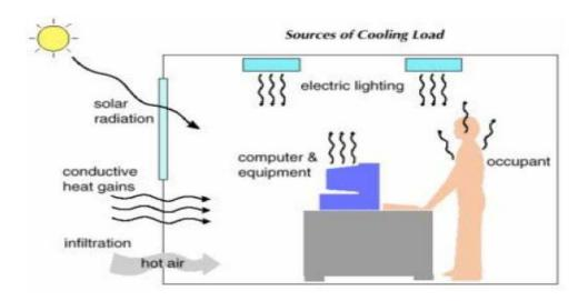
Fig 1.1 sources of heat gain
