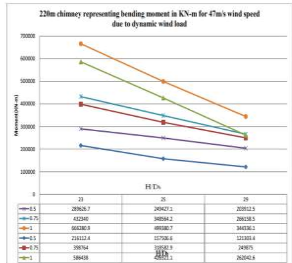
Fig5.3: Moments due to wind analysis for 220 m RCC Chimney for 47m/s wind speed
