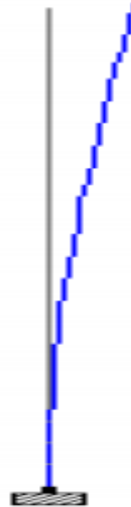
Fig 4.2 STAAD model of Chimney using Line/Beam elements
