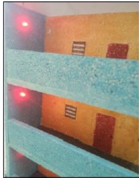
Fig. 4.5 Red LED is turned ON once the waste reaches the level of 70% full.
