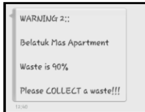
Fig. 4.6. The second notification SMS sent by the system, indicating that bin is at least 90% full and the garbage needs to be collected immediately
