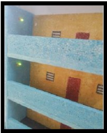
Fig. 4.3 GREEN LED is turned ON once the waste reaches the level of 70% full.
