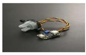
The **arduino turbidity sensor** detects water quality by measuring the levels of turbidity. It uses light to detect suspended particles in water by measuring the light transmittance and scattering rate, which changes with the amount of total suspended solids (TSS) in water. As the TTS increases, the liquid turbidity level increases.
