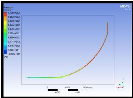
Fig 10:-Pressure in Model 1 using air
