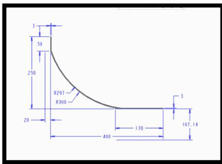
Fig 4:-Drafting of model 1 with  $t_2/b_2 = 0.028$  for original configuration
