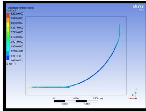
Fig 12:-Turbulence kinetic energy in Model 1 using air
