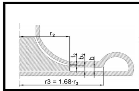
Fig 2: – A schematic view of the flow path and pinch.
