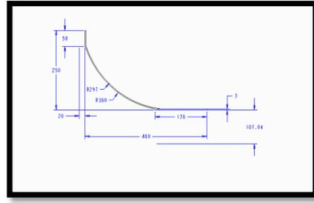
Fig 6:-Drafting of model 5 with  $t_2/b_2 = 0.028$  for 10% pinched configuration
