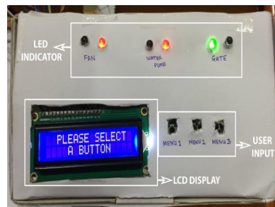
Figure 2: Control Panel of Aquaponic System
