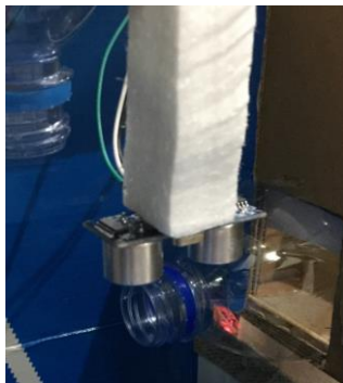
Figure 6: Ultrasonic sensor mounted above the fish tank
