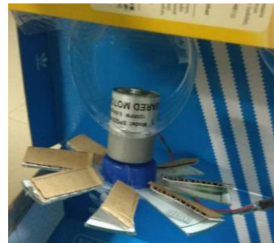
Figure 8: DC motor as fan to increase aeration of fish tank
