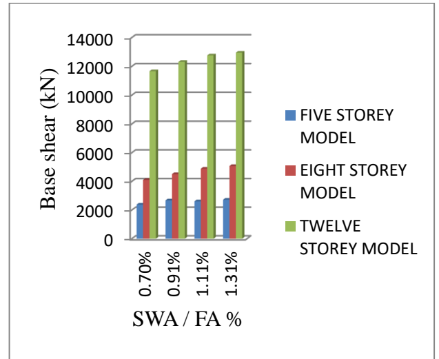
Fig 7. SWA / FA (%) vs. Base shear of five, eight and twelve storey – Seismic force in Y- direction
