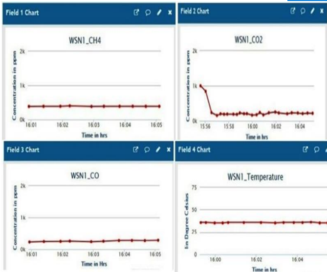
Figure 8: wireless sensor node 1 gas levels displayed on IoT fields
