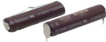
Figure.6: a) CO gas sensor module
