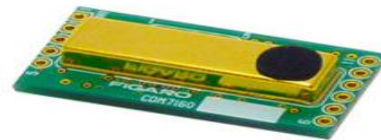
Figure.5: CDM7160 CO 2 gas sensor
