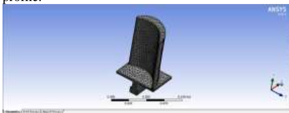
Fig Meshing of first stage rotor blade
