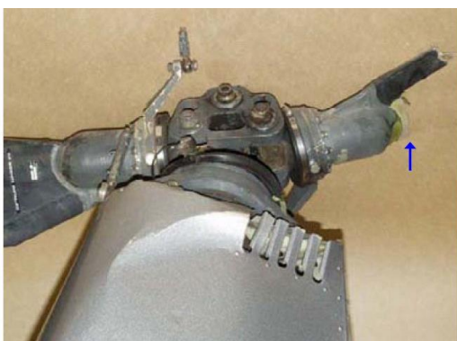
Fig. The fracture location (arrowed) is located at rotor station (RS) 10.35, the location of the inboard bolt hole in the fitting to spar joint.
