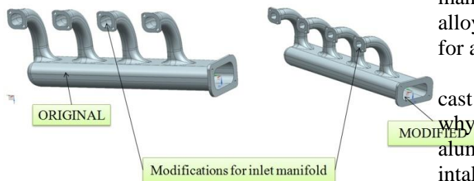
Fig. shows Comparison of original and modified inlet manifold models
