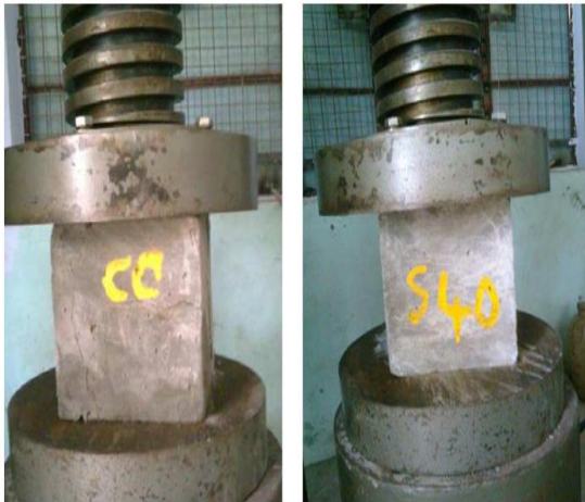
Figure 6.1 Compression test on CC and S40 specimens
