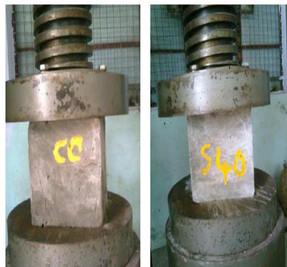
Figure 6.1 Compression test on CC and S40 specimens
