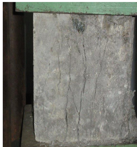
Figure 3.16 Concrete cube at failure
