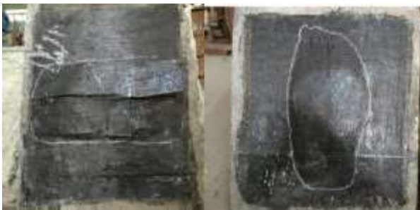
Fig 9: Failure pattern of CFRP wrapped rehabilitated slab.
