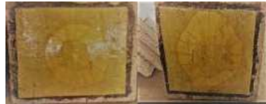
Fig 11: Failure pattern of AFRP wrapped rehabilitated slab.
