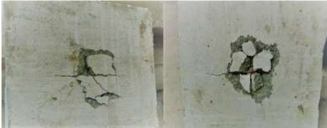
Fig: 7: Failure pattern of control slabs
